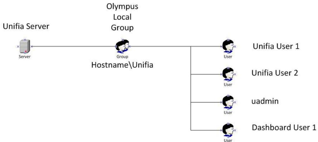
It is recommended if a facility moves from a workgroup environment configuration to a domain configuration, that the local 'Unifia' group on the application server is cleaned up so only the active directory group and the 'uadmin' user are present:
