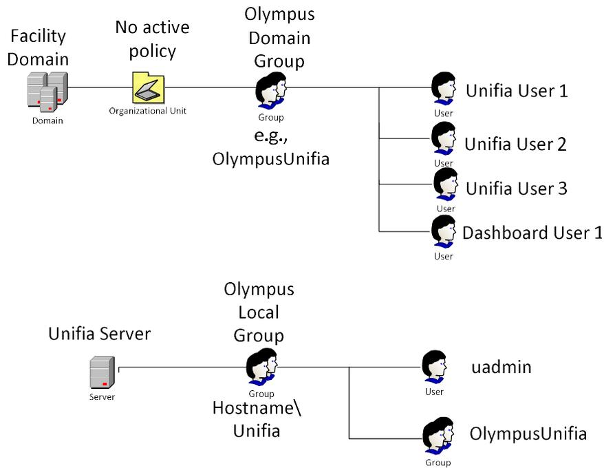
It is possible for the application to be in a workgroup environment. In that configuration, all users are created on the application server and must be placed in the 'Unifia' group as shown below.
