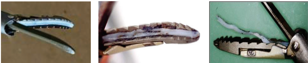
Figure 2. Example of THUNDERBEAT Probe in accordance with specifications (Left), Tissue Pad Deformation (Center), Tissue Pad Detachment (Right)
