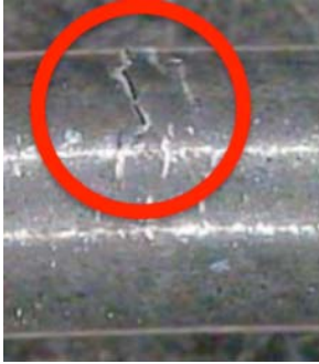
Cracking of the insertion tube
