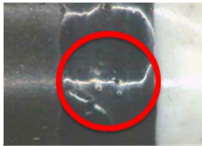
Bubbling of adhesive at bending section cover
