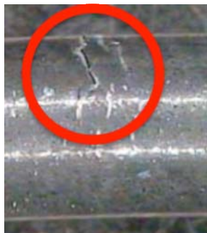
Cracking of the insertion tube
