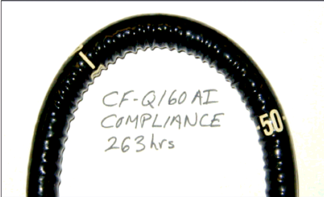
FIGURE 1. This insertion tube was immersed continuously in Compliance™ for 263 hours at room temperature. The deterioration that caused an early failure of the insertion tube has become even more obvious. The black polymer layer of the insertion tube is swollen and has loosened from the metal mesh below. The white markings have yellowed. The insertion tube has lost its normal elasticity and handling characteristics.
