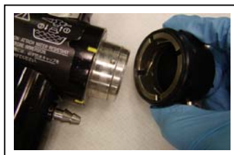
Fig. 2. Water resistant cap removal from Olympus videoscopes
