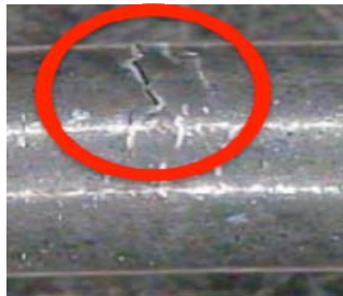
Cracking of the insertion tube
